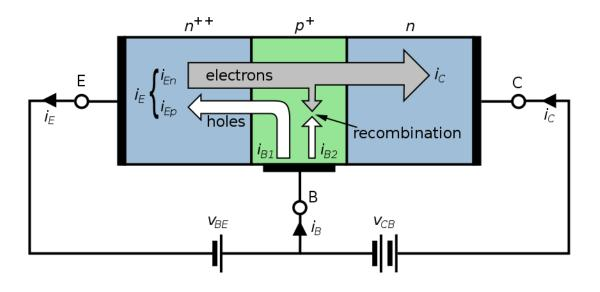
A BIPOLAR JUNTION TRANSISTOR (BJT) IS A THREE TERMINAL SEMICONDUCTOR DEVICE IN WHICH THE OPERATION DEPENDS ON THE INTERACTION OF BOTH MAJORITY AND MINORITY CARRIERS AND, HENCE THE NAME BIPOLAR. THE BJT IS ANALOGOUS TO A VACUUM TRIODE AND IS COMPARATIVELY SMALLER IN SIZE. IT IS USED IN AMPLIFIER AND OSCILLATOR CIRCUITS, AND AS A SWITCH IN DIGITAL CIRCUITS. IT HAS WIDE APPLICATIONS IN COMPUTERS, SATELLITES AND OTHER MODERN COMMUNICATION SYSTEMS.
