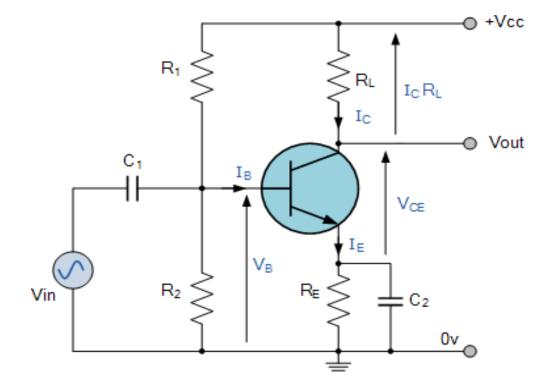
IN THIS CIRCUIT, AN NPN TRANSISTOR IS USED IN CE CONFIGURATION. HERE Vbb SUPPLY WILL FORWARD BIAS THE EMITTER- BASE JUNCTION AND Vcc SUPPLY COLLECTOR-BASE JUNCTION. THIS BIASING ARRANGEMENT MAKES THE TRANSISTOR TO OPERATE INN THE ACTIVE REGION. THE MAGNITUDE OF THE INPUT AC SIGNAL VI ALWAYS FORWARD BIAS THE EMITTER-BASE JUNCTION REGARDLESS OF THE POLARITY OF THE SIGNAL.
