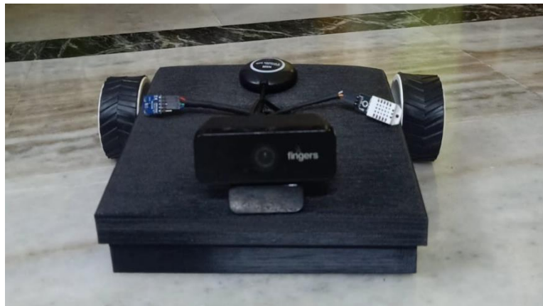
Fig 3: An exterior view of the "AuraHeat" autonomous micro-climate rover prototype, showcasing its sensor suite and computer vision webcam.
